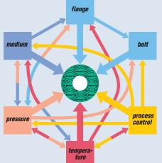
Maximum temperature and pressure values alone can not define a material's suitability for an application. These limits are dependent upon a multiplicity of factors as shown in the diagram opposite. It is always advisable to consider these factors when selecting a material for a given application.
